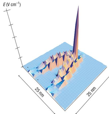
**Figure 2** The electric field provided by the spaser described in ref. 1. Mode electric-field amplitude,  $E$ , is plotted over the surface of a V-shaped silver nanorod configuration that acts as a spaser resonator.
