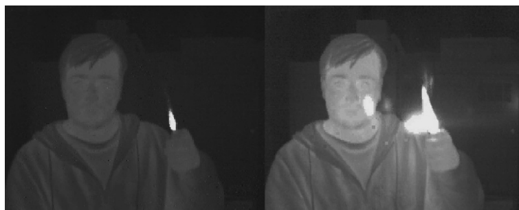
Fig. 18. An image taken with the 320 \times 256 pixel co-registered simultaneously readable MWIR:LWIR dualband QWIP camera. The person in this image is holding a cigarette lighter. The cigarette lighter produced lots of hot \text{CO}_2 gas. So, flame in MWIR image looks broader due to re-emission of infrared signal in 4.1\text{--}4.3\ \mu\text{m} band by the heated \text{CO}_2 gas produced by the cigarette lighter. Whereas, heated \text{CO}_2 gas does not have any emission line in the LWIR ( 8\text{--}9\ \mu\text{m} ) band. Thus, LWIR image shows only thermal signatures of the flame. The hot cigarette lighter flame produced a lot of MWIR signal, so it reflects off from the lens and face.
