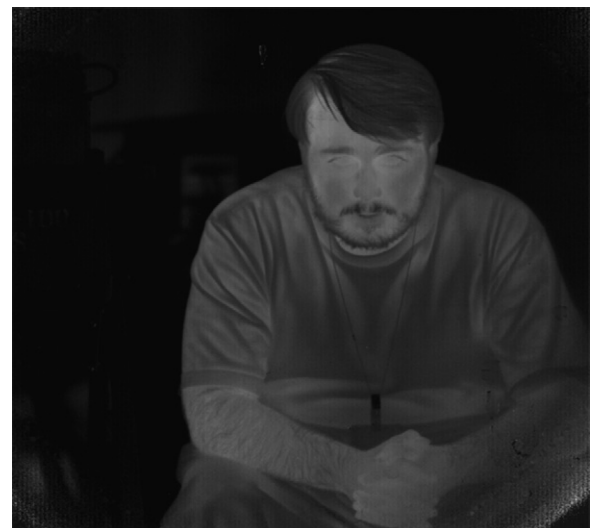
Fig. 13. One frame of video image taken with the 9 \mu\text{m} cutoff 1024 \times 1024 pixel QWIP camera.
