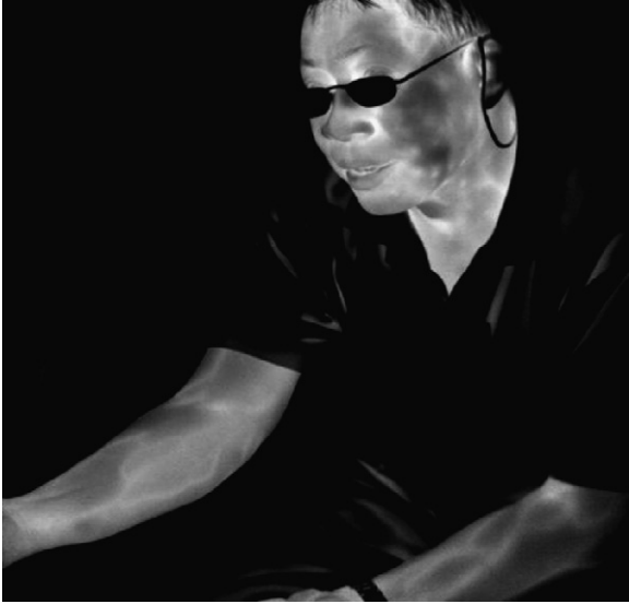
Fig. 8. One frame of video image taken with the 5.1\ \mu\text{m} cutoff 1024 \times 1024 pixel QWIP camera.
