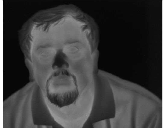
Fig. 10. An image taken with the first 640 \times 512 pixels QDIP LWIR focal plane array camera.
