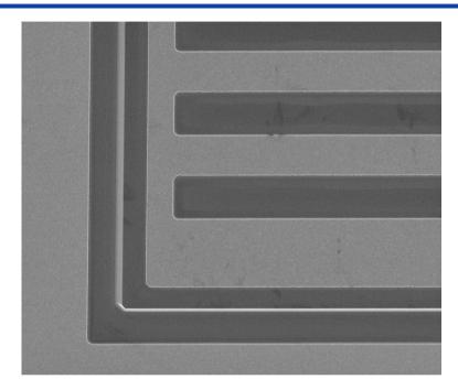
Samples were processed into square shaped mesas of different sizes (1000, 710, 500, 350, 250, 180, 130  $\mu$ m) using standard photolithography, wet etching with H<sub>2</sub>SO<sub>4</sub>:H<sub>2</sub>O<sub>2</sub>:H<sub>2</sub>O and lift-off procedure.
