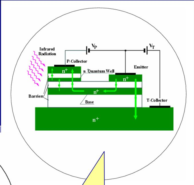
QWIP-HET – unipolar Darlington infrared phototransistor, 1997
