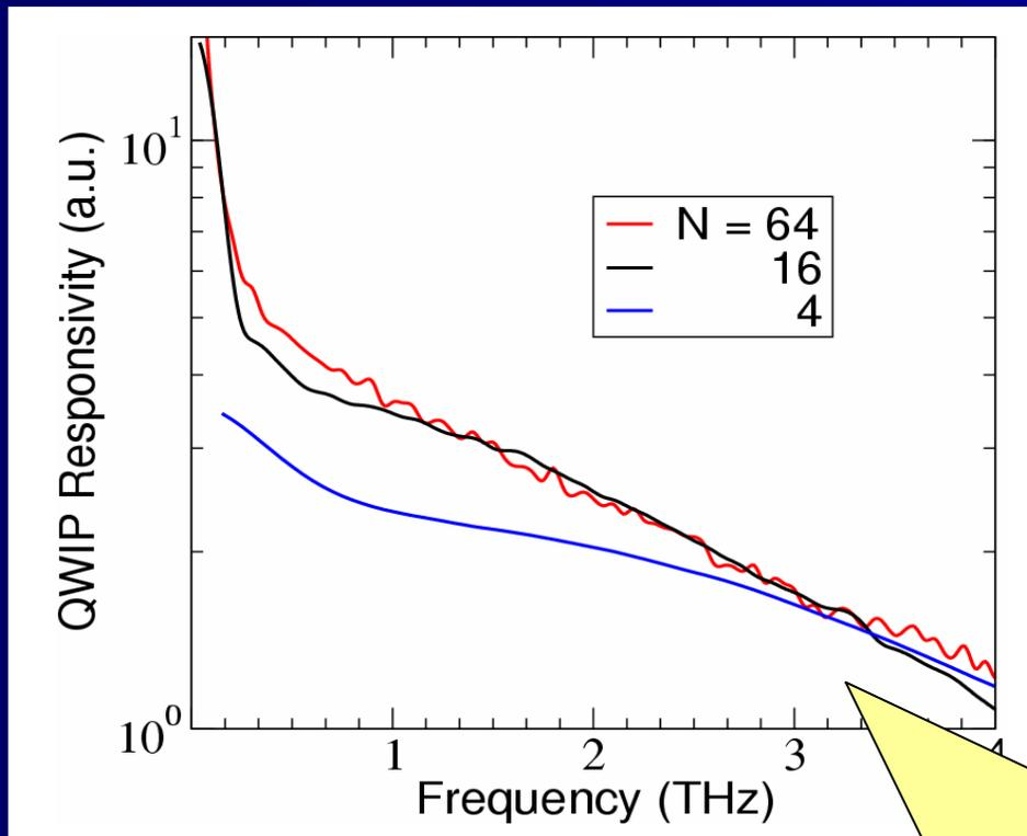
Long tails correspond to relatively strong QWIP response at THz frequencies – consequence of **velocity overshoot** of just photoexcited electrons
