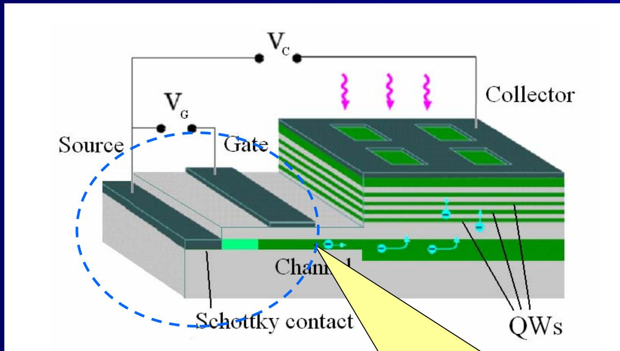
Resonant plasma oscillations can lead to relatively large rectified component of net current
