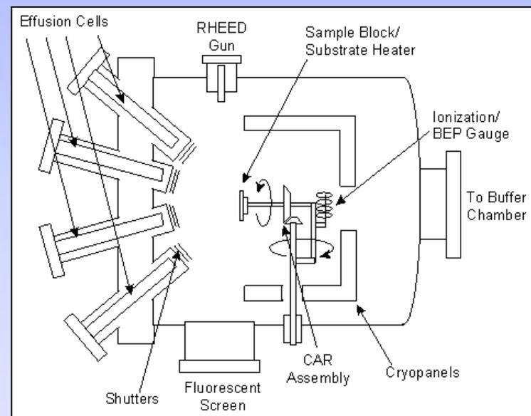
Schematic of an ultra high vacuum MBE chamber
