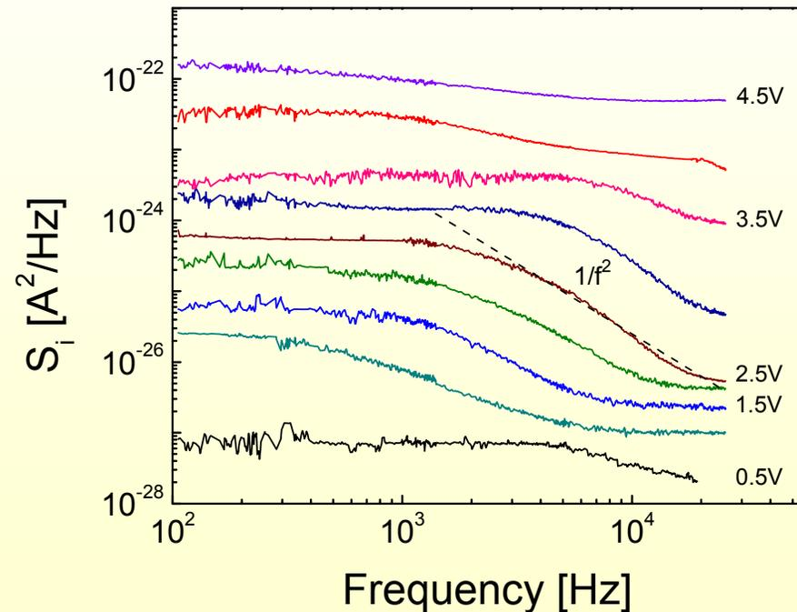
Dark current noise spectrum for different positive voltages at 77K.
