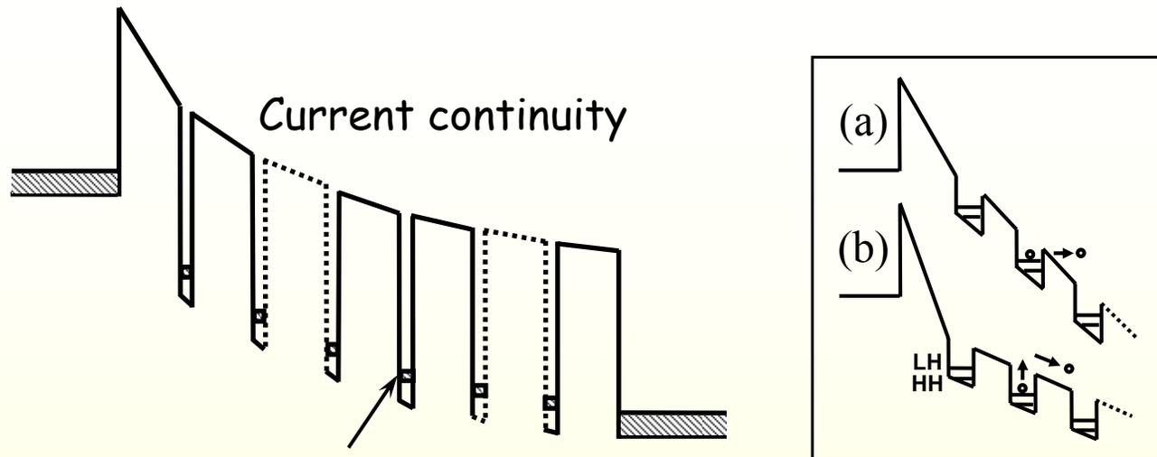
Possible different resistivity states, characterized by different electric field distributions.
