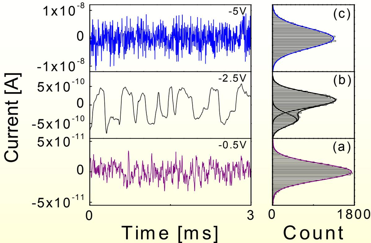
Time traces of the dark current and corresponding noise amplitude distributions for different bias voltages at 77 K.
