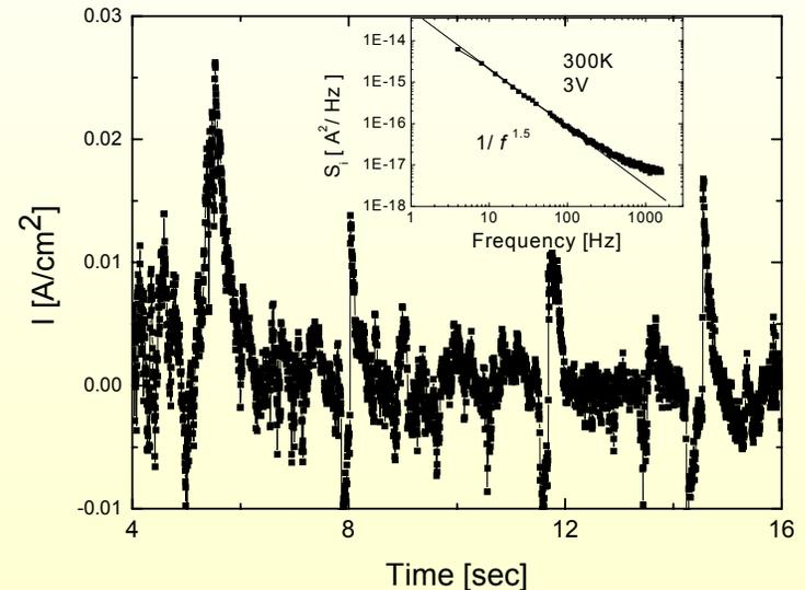
Crackling avalanche noise as measured in transport through a nanodots system
