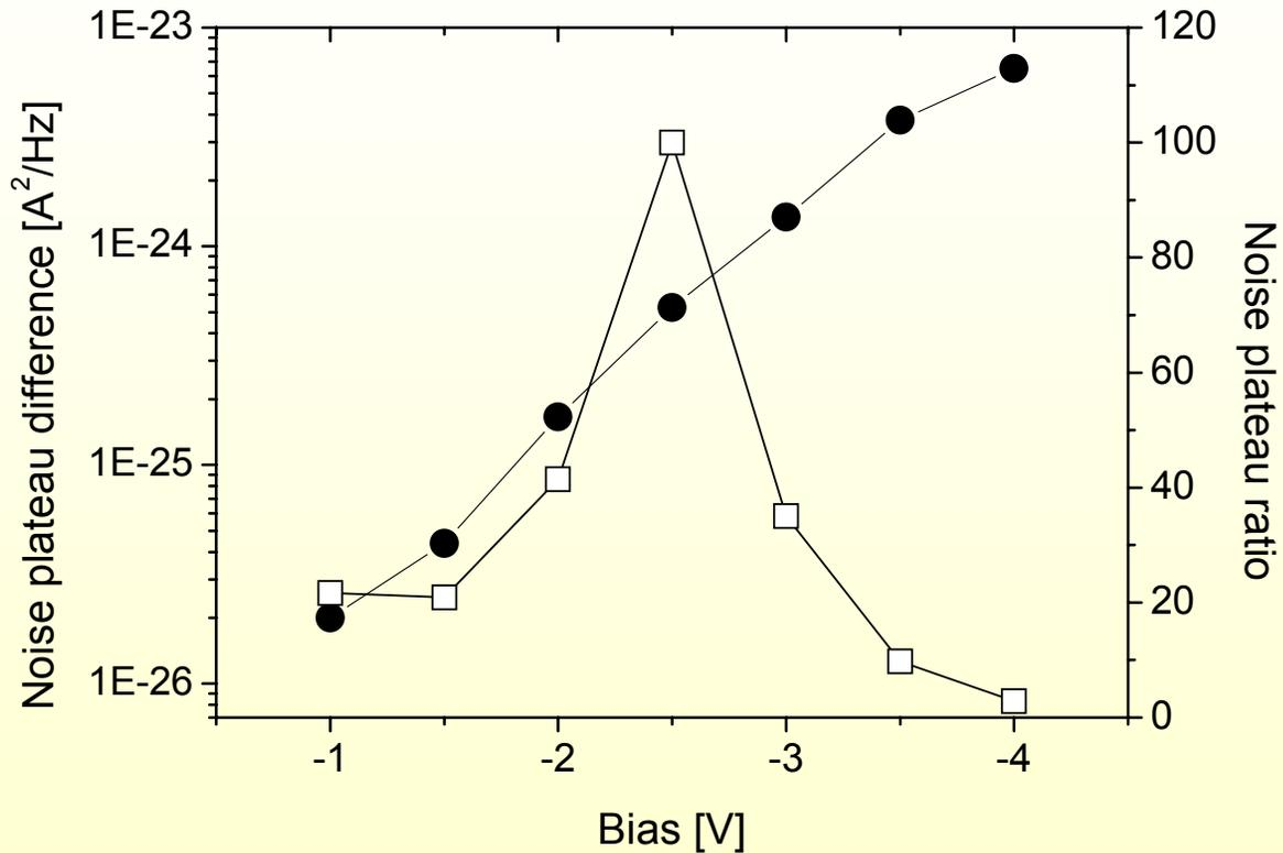
Bias dependence of the RTN amplitude (solid circles) and ratio between the RTN plateau to the GR plateau (open squares).
