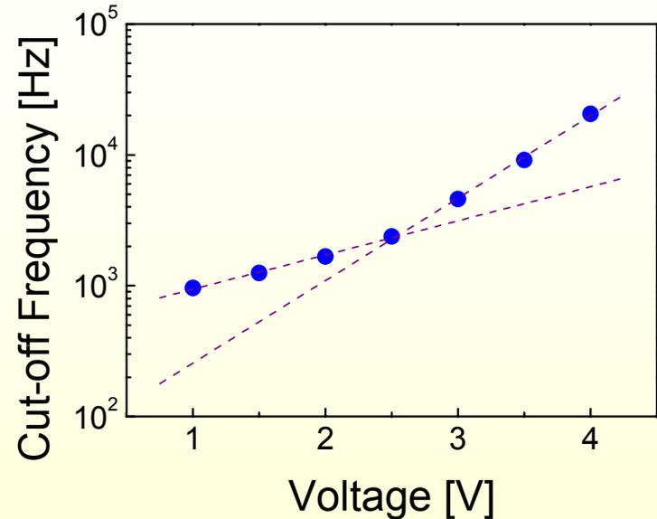
Bias dependence of the cut-off frequency determined from the spectra.
