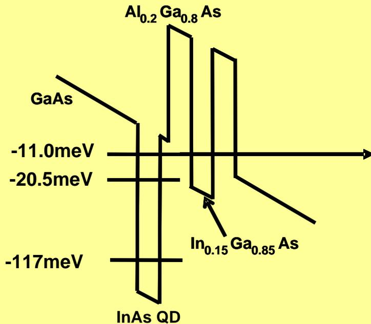
Schematic diagram of conduction band of terahertz T-QDIP.
