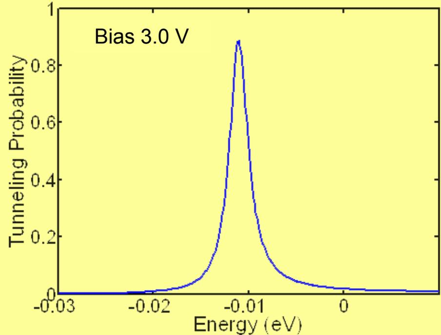
Calculated tunneling probability of THz T-QDIP as a function of energy.
