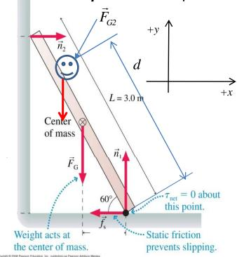
As sketched below, a ladder (L = 3.0 m & mass = 15 kg) leans against a frictionless wall at the angle  $\theta = 60^{\circ}$ . If the coefficient of static friction between the ladder and the floor is  $\mu_k = 0.4$ , how far up the ladder (d) can a 75 kg person climb before it begins to slip on the floor?
