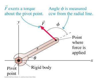
Work = ( $F_{effective}$ ) (distance) =  $F_{//}d$ = Fdcos $\theta$ Torque = ( $F_{effective}$ ) (lever arm) =  $F_{\perp}d$ =Fdsin $\phi$
