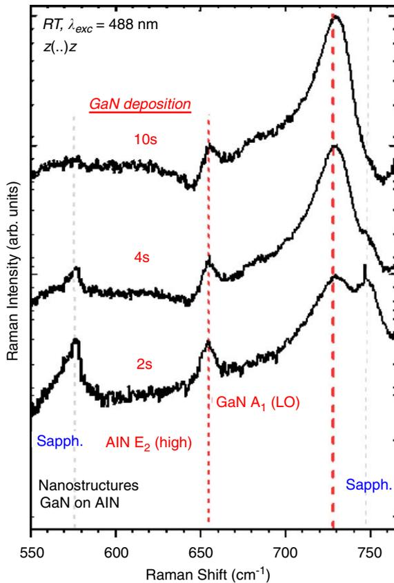
Fig. 4. Raman spectra of GaN nanostructures for different GaN deposition times. The intensity of the GaN modes increases with the deposition time.
