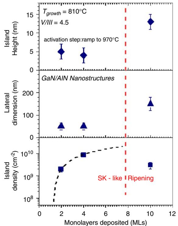
Fig. 3. GaN/AlN nanostructure density and dimensions as a function of the monolayers deposited. Two critical thicknesses are observed at approximately 2 and ~8 MLs.
