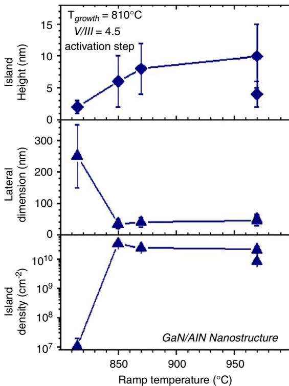
Fig. 2. Two-step growth process: GaN/AlN nanostructure density and dimensions as a function of the maximum temperature applied for the activation step.
