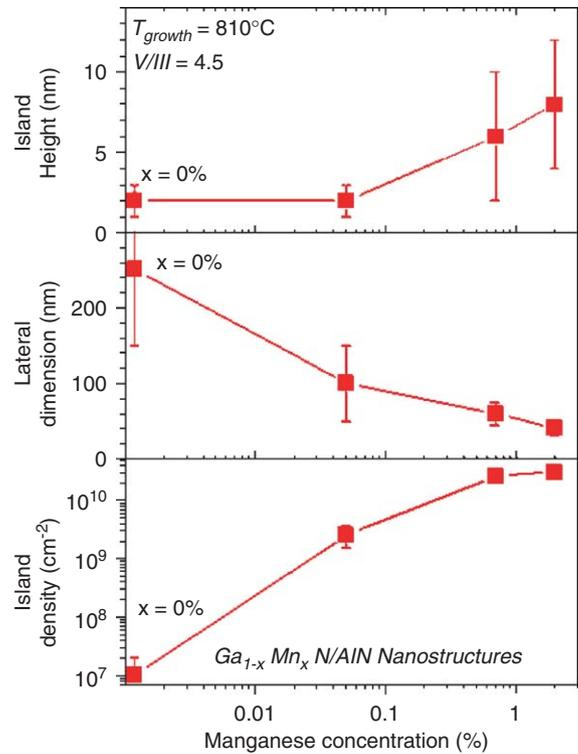
Fig. 5. GaMnN nanostructure density and dimensions as a function of Mn concentration. The presence of Mn enabled the formation of nanostructures without an activation step.
