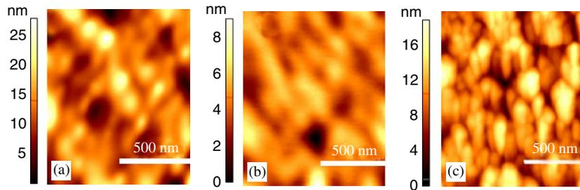
Fig. 1. (a) GaN/AlN nanostructures obtained at a V/III ratio of 20 with silane incorporation. (b) 2D growth at a V/III ratio of 4.5 without silane. (c) Sample grown under the same conditions as in (b), but with an activation step including a temperature ramp up to 970 °C applied after the GaN deposition. The activation step enhances 3D growth.
