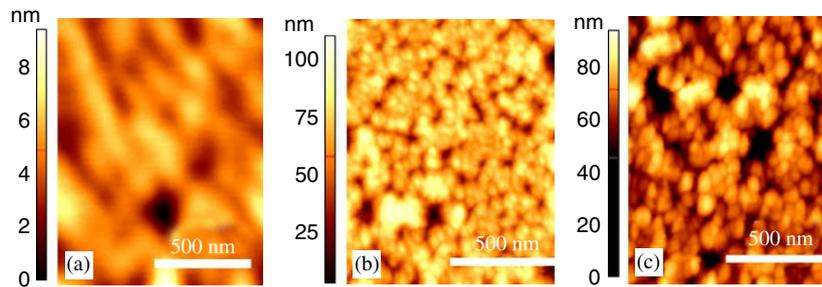
Fig. 6. (a) 0% Mn shows 2D like behavior. (b) Mn incorporation enhances nucleation and results in 3D growth, resulting in increased island density and reduced lateral dimension. (c) Activation step above 880 °C in GaMnN nanostructures leads to ripened islands.
