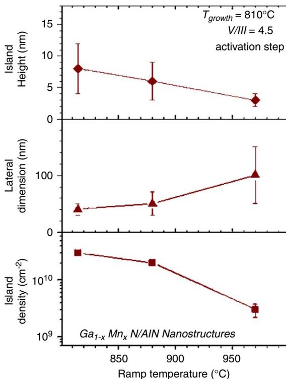
Fig. 7. GaMnN containing 2% Mn is activated at different temperatures. Activation steps with temperatures above 880 °C applied to GaMnN nanostructures lead to a ripening process providing larger islands and smaller densities.
