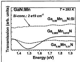
Figure 4: Transmission spectra of Ga1-xMnxN with varying Mn concentrations. In addition, a transmission spectrum of a co-doped Ga<sub>1-x</sub>Mn<sub>x</sub>N:Si sample is shown. The spectrum of the Si co-doped sample is vertically shifted for clarity.
