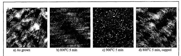
Figure 2: Atomic force microscopy images from the Ga<sub>1.x</sub>Mn<sub>x</sub>N (x=0.015) terminated (a-c) and GaN terminated (d) MOCVD grown Ga<sub>1-x</sub>Mn<sub>x</sub>N samples under various annealing conditions. All scans are 10 µm x 10 µm. RMS roughness values from left to right are: top row: 5.68 Å, , 5.94 Å, 7.71 Å, and 6.88 Å,
