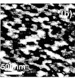
Figure 7: AFM picture of GaN nanostructure (a) and GaMnN nanostructures (b) on AlN. The height of the nanostructures was 40 and 15 nm, respectively.
