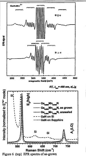
Figure 6 (top) EPR spectra of as-grown Ga<sub>0.985</sub>Mn<sub>0.015</sub>N<sub>98</sub>Mn<sub>0.02</sub>N:Si recorded in magnetic fields parallel and perpendicular to the c-axis at 5K. The presence of Mn<sup>2+</sup> ions in GaN is unambiguously proven by the hyperfine resonances. (bottom) Raman spectra of MOCVD-grown GaN epilayers with different Mn concentrations and sample preparation. For comparison, GaN epilayers grown on sapphire and on Si substrates are also shown.
