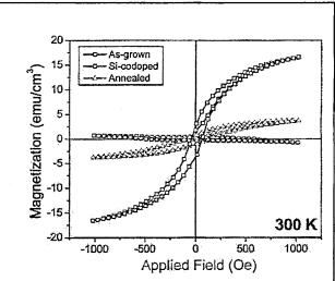
Figure 3: Magnetization vs applied field taken at room temperature for as-grown Ga<sub>1-x</sub>Mn<sub>x</sub>N (x=0.01), and samples following 800°C anneal and codoping with high levels of silicon (~1e20). Note the decreased magnetic signature with annealing or silicon codoping
