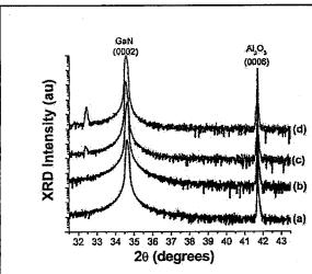
Figure 1. XRD diffraction scans of (a) undoped GaN template layer, (b) as-grown MOCVD GaMnN layers, (c) MOCVD grown GaMnN layer annealed at 700°C, and (d) MOCVD grown GaMnN layer annealed at 900°C
