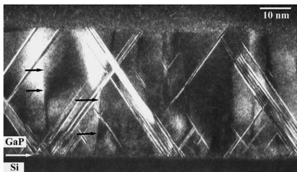
Fig. 1. A DF-TEM micrograph obtained using the (002) reflection, of a GaP epilayer on (001) Si after 500s of growth at 420 °C. Notice the contrast change across boundaries indicated by arrows.
