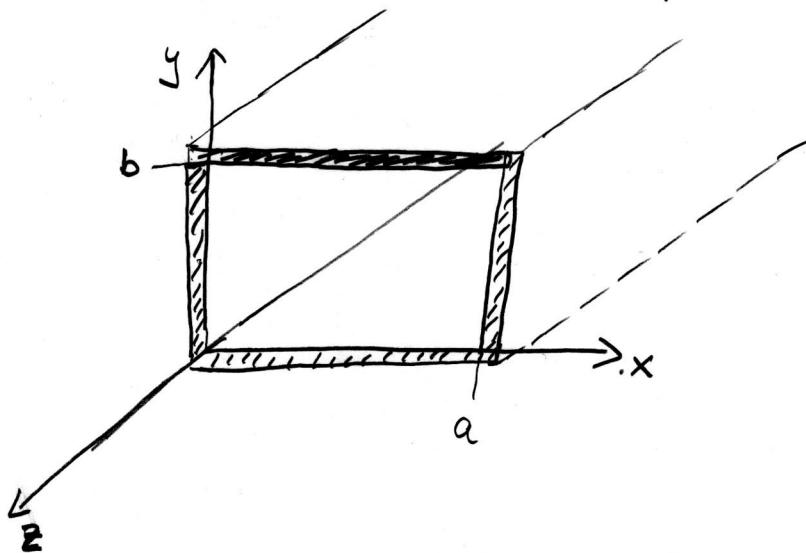
Assume a rectangular conductor with the inside length  $a, b$  in  $x$ - and  $y$ -direction respectively.
