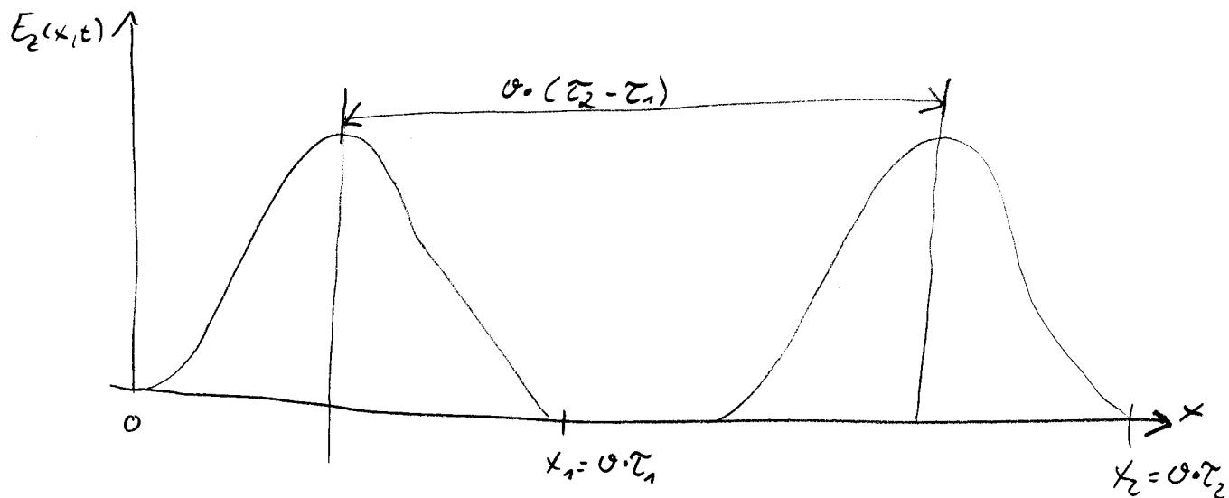
EM-wave propagation: damped waves in conducting media.
