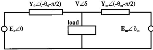
FIG. 1. The modified electric power-system model of Wang and Abed. The model consists of two generators with voltages  $E_0$  and  $E_m$ , and a load consisting of an induction motor and a  $PQ$  load in parallel.
