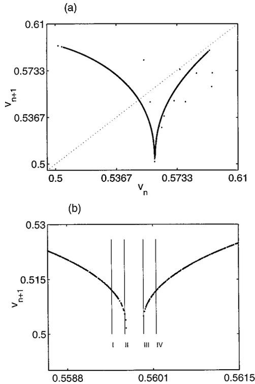
FIG. 4. The return maps constructed from the local minima of  $V(t)$ : (a) after the crisis at  $Q_1 = 2.5603784$ ; and (b) a blowup part of (a) near the cusp. There is an escaping gap, enclosed between lines II and III, in the middle through which a trajectory asymptotes to the state with  $V=0$  (voltage collapse). Two regions to the left (I–II) and the right (III–IV) of the gap are the regions from which a set of target points are chosen for control.
