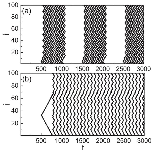
Fig. 3: Effect of on-off switch with the initial network of 9 directional links from the source node 1 to the nodes 10, 20,  $\dots$ , 90. A new link will be added at the time  $t = 500$ , removed at  $t = 1000$ , added again  $t = 1500$ , removed again at  $t = 2000$  and so on. (a) and (b) represent the cases of adding the new link from the source node 1 to nodes 5 and 33, respectively.
