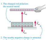
2. The nearby negative charge is attracted to the rod more strongly than the distant positive charge is repelled, resulting in a net upward force.
