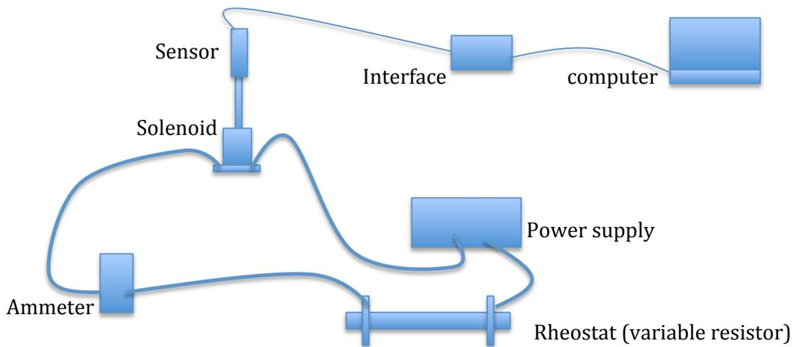
8. Power supply is set around 5.0V for you and adjust the rheostat until the current indicated by the ammeter is 0.25 A. Place the magnetic sensor as shown above and make sure that aligns with the axis of the solenoid. Insert the probe about one inch into the solenoid and read the measurement. With trial and error find out the maximum reading for recording. Record the reading below with units.
