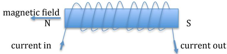
You are given a solenoid and it is an electromagnet. Carefully observe how it is made. An insulated wire is wrapped around a hollow metallic cylinder. When a current flows through the wire the solenoid becomes an electromagnet. In this experiment you want to investigate the strength of the magnetic field inside the solenoid as the current is varied.
