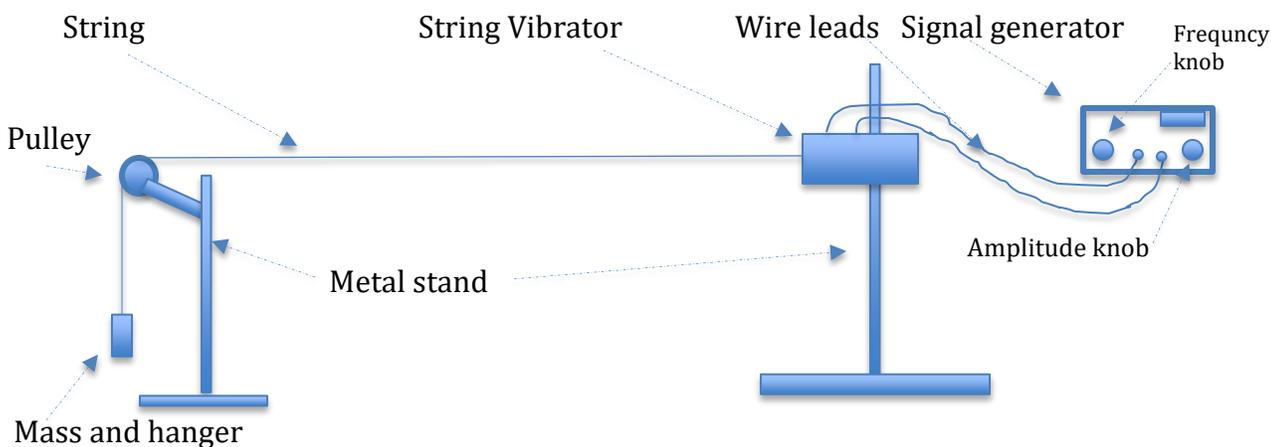
10. Now slowly increase the frequency of the signal generator starting at 0 Hz and carefully observe the formation of standing waves which have a good node at the vibrator end. Once you reach such a frequency, fine tune it with fine frequency adjustment. Complete the observation/measurement chart below.
