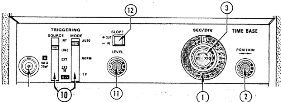
Time base front panel controls and connectors.
