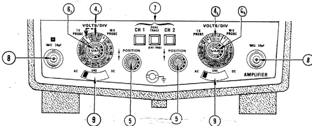
Vertical amplifier front panel controls.
