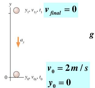
$$v_{t} = v_{0} - gt$$
