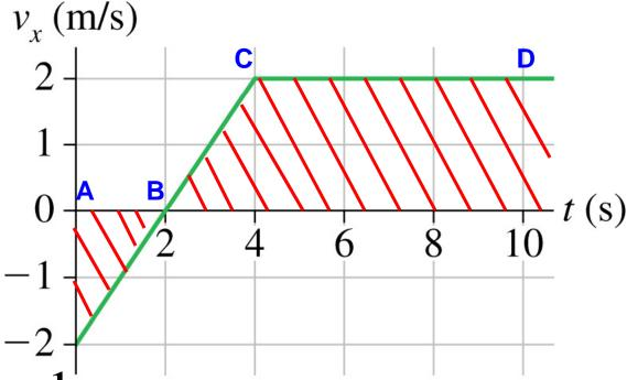
$$x_{A-B} = x_B - x_A = \int_{t_A}^{t_B} v(t)dt = -\frac{1}{2} 2 \cdot 2 = -2m$$
