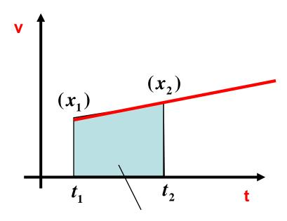
$$x_{2-1} = x_2 - x_1 = \int_{t_1}^{t_2} v(t)dt$$
