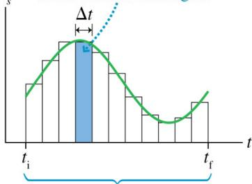
During the interval  $t_i$  to  $t_f$ , the total displacement  $\Delta s$  is the "area under the curve."
