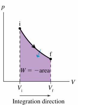
As the piston moves dx, the external force does work  $F_{ext} dx$  on the gas.
