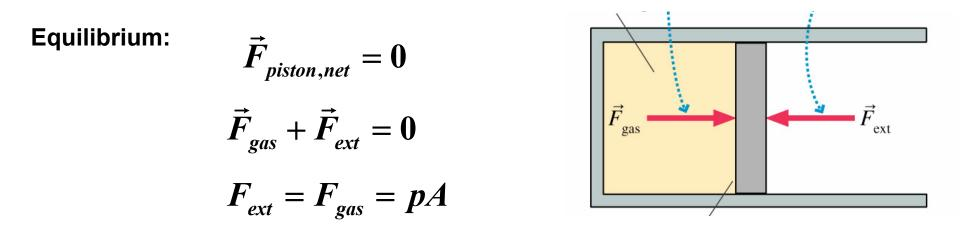
We move piston (by changing a little bit external force) very slow, so the velocity of the piston is almost 0. Then all the time we have condition
