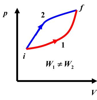
Specific heat depends on the path For both processes (1 and 2) the initial temperature and the final temperature are the same, but the work different.
