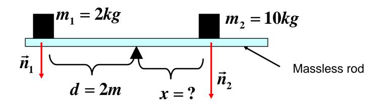
Two forces (which can results in rotation) acting on the rod
