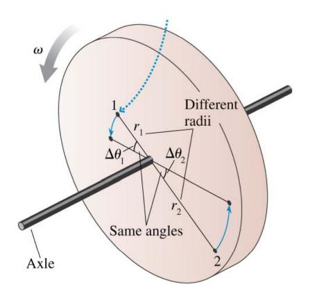
The relation between angular velocity and angular acceleration is the same as the relation between linear velocity and linear acceleration
