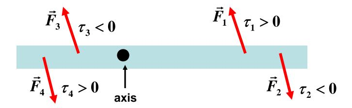
The net torque is the sum of the torques due to all applied forces:
